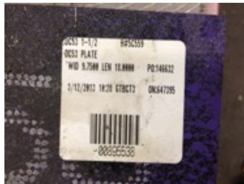
Anytime a piece of steel is cut in our facility it is first scanned to determine that the correct material has been selected. The steel is then cut to the customers required size, repainted to correspond with the correct color code, the material is measured (both the piece for the customer and the remaining material to be put back into stock), and a bar code is generated for both the put back material and the customers piece.
